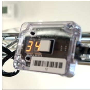
Position Displays guide items into each tote position on a cart
