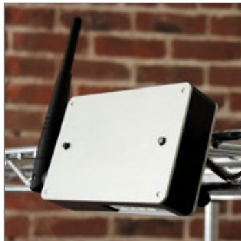
Aisle Controllers drive shelf lights
