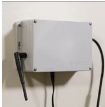
Site Master Controller wirelessly drives Aisle and Cart Controllers
