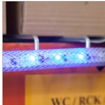
Shelf Lights display 7 colors, each guiding a different worker
