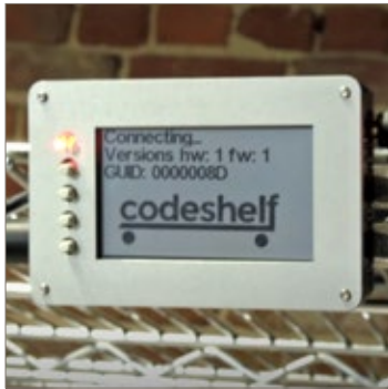
Cart Controller drives Position Displays
